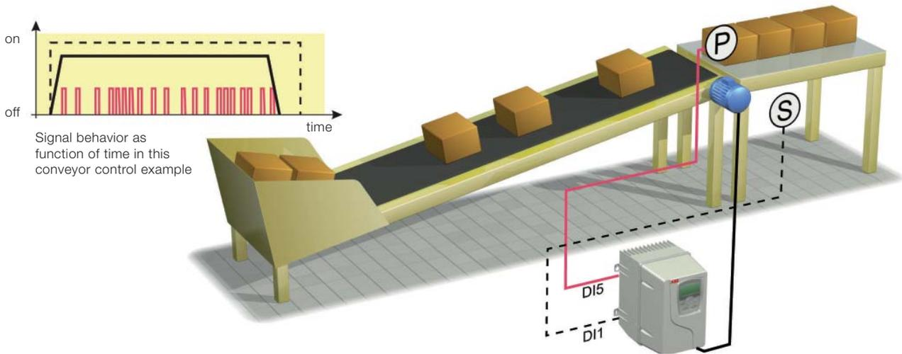
The ACS355 drives have many solutions for common challenges. The following example explains how the COUNTER STOP function operates within a conveyor unloading routine. The function stops the conveyor after a predefined number of boxes have passed the sensor.
